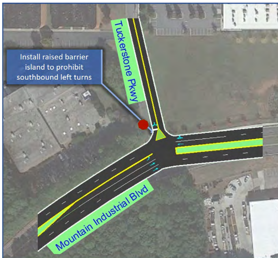
Figure 22: Proposed Improvement at Mountain Industrial Boulevard and Tuckerstone Parkway – Right In, Right Out at Tuckerstone
