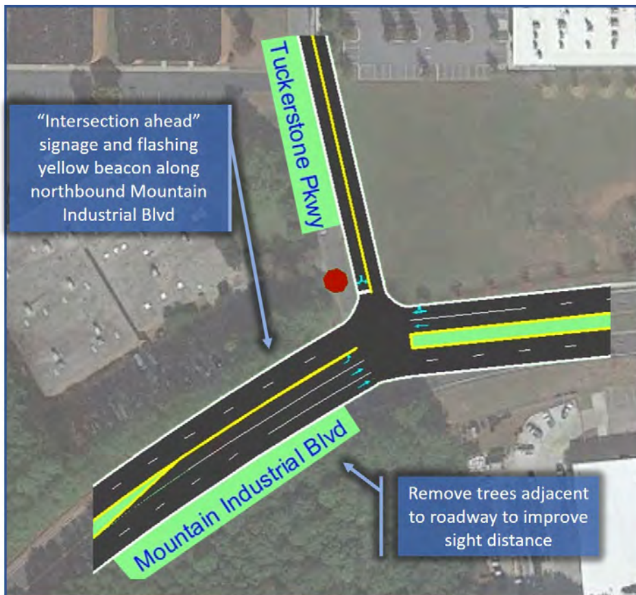
Figure 20: Proposed Improvement at Mountain Industrial Boulevard and Tuckerstone Parkway – Clear Cut and Signalization
