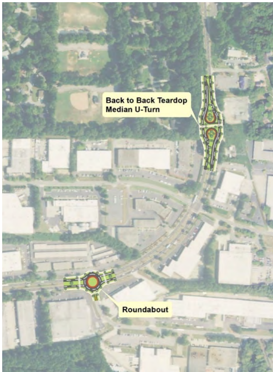
Figure 28: Mountain Industrial Boulevard and N. Royal Atlanta Drive/S. Royal Atlanta Drive Improvements
