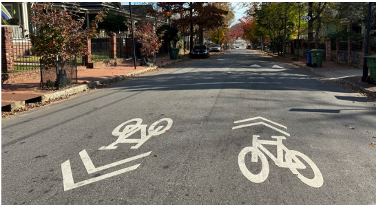
A neighborhood greenway in Atlanta is indicated with shared lane markings and speed bumps.
